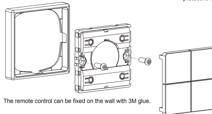
The remote control can be fixed on the wall with 3M glue.
