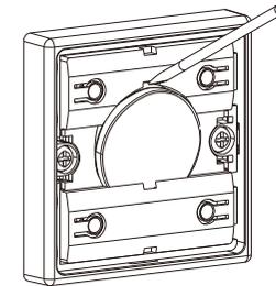
**Step 1:** Remove the buttons from the switch with hand or a tool.
